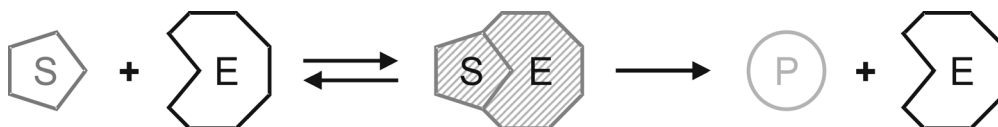
Figure 1.1: Reaction scheme of an enzyme-catalyzed conversion of the substrate S to the respective product P.
